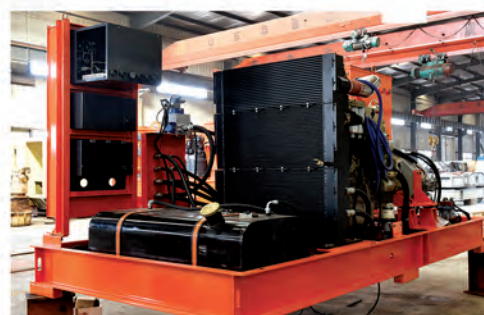
动力系统装配 Power System Assembly
