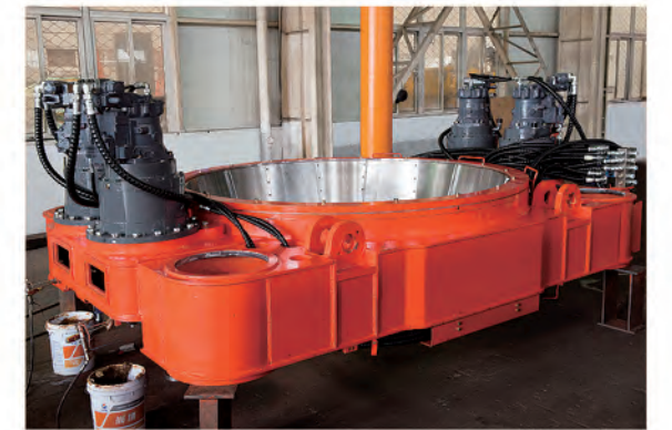
传动轴箱安装 Transmission box Installation
