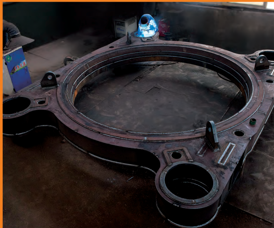
结构件焊接 Structures Welding
