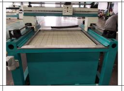
10. Use soft cover which can protect linear guider and ball screw better.
