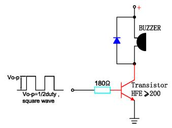
The base current Ib should high enough so that it saturates the collector current of the transistor with the CB load.
