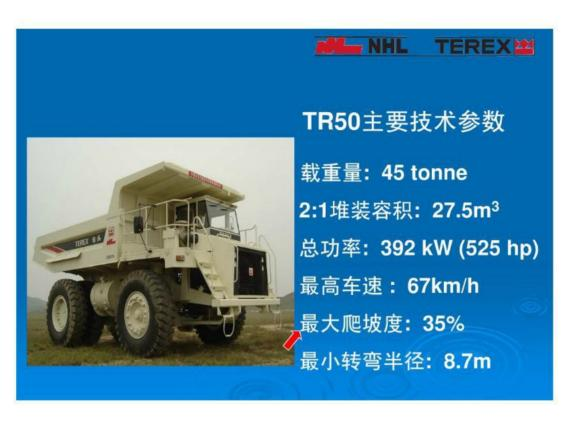
Cummins turbo charged, aftercooled engine Smooth shifting, electronically-controlled transmission Non-wearing hydrodynamic retardation High visibility cab with de-luxe interior
