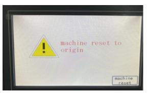
Press "machine reset" to rest the machine actions.
