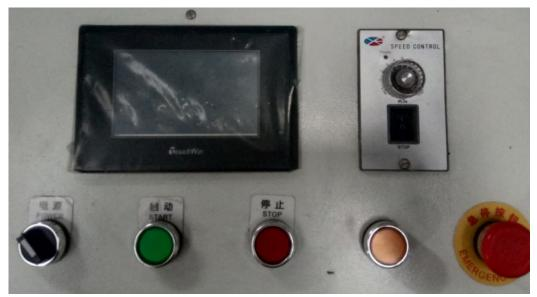
After the device is powered on, press the <power switch> on the machine and it will turn red after being pressed.
