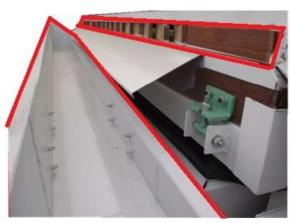
Air Volume Adjusting Handles (adjust air volume according material's specific weight)
