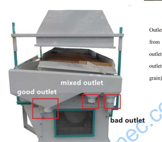
Outlets of gravity separator, from left to right is good outlet (heavy grain), mixed outlet and bad outlet (light grain)
