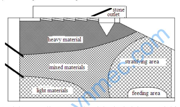
The vibration deck is supported by an eccentric drive which makes the deck to move in high frequency and low amplitude. And the heavy materials will move up towards higher position of deck, while light materials move down towards lower position of deck. And in this process also generate of mixed materials which will be discharge from middle outlet .At the same time, some heavier gravity like stones will be discharged separately.
