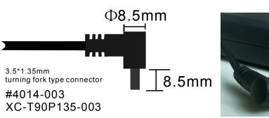
recommended plug for heating wears connecting to this battery.
