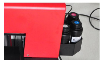
ink bottle tray tray for the ink rotate bottles
