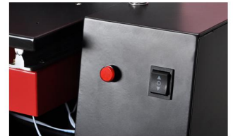
Up/down button Up and down the tray
