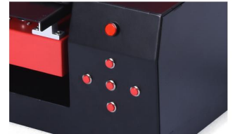
Up/down button Up and down the tray
