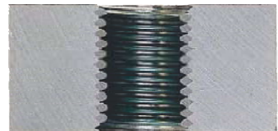
Steel screw screwed into the bottom section diagrammatic sketch
