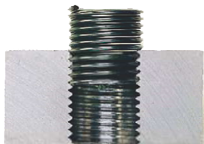
Steel screw screwed into the bottom section of the real contraction
