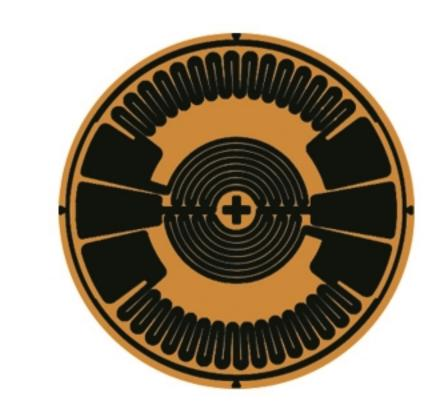
Resistance type strain gauge is sensitive component, which uses resistance-strain effect and converts strain quantity of test piece into resistance change quantity, is the widest strain test component at present, and is mainly used in weighing/force measuring field.
