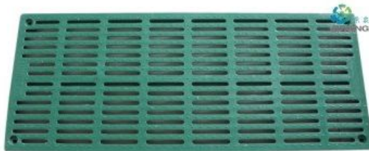
Name:BMC Slat Floor For Piglet Type:RQLF003-1100*450*35(Classic) Gap:13mm/11mm
