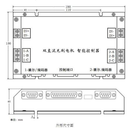
**Note:** The bottom of controller shell has  $4*\Phi5mm$  holes for installation and fixing, and installation can be conducted in the horizontal direction.
