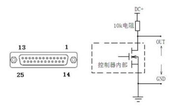
The controller provides 6-way (8-way at most) digital output. The terminals are the MOS tube open-drain, the universal output amplitude is 24V 1A, and the maximum output is 40V 1A. In practical use, it is essential to connect a 10k pull-up resistor (as appropriate), as shown in the figure. For the digital output of every way, MOS tube breakover or turn-off can be chosen according to a preset event status.
