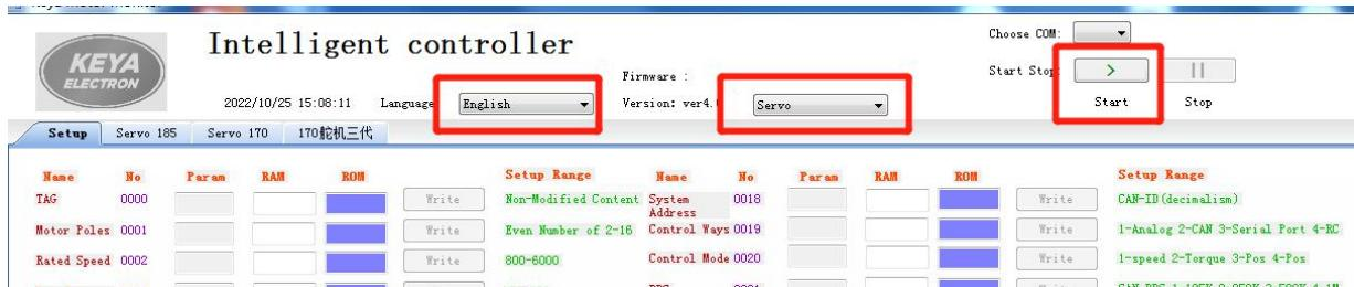
4.1.2.3 Open the configuration interface, select “170 三代” and click the “Connect” button in the lower left corner to establish a connection between the software and the controller.
