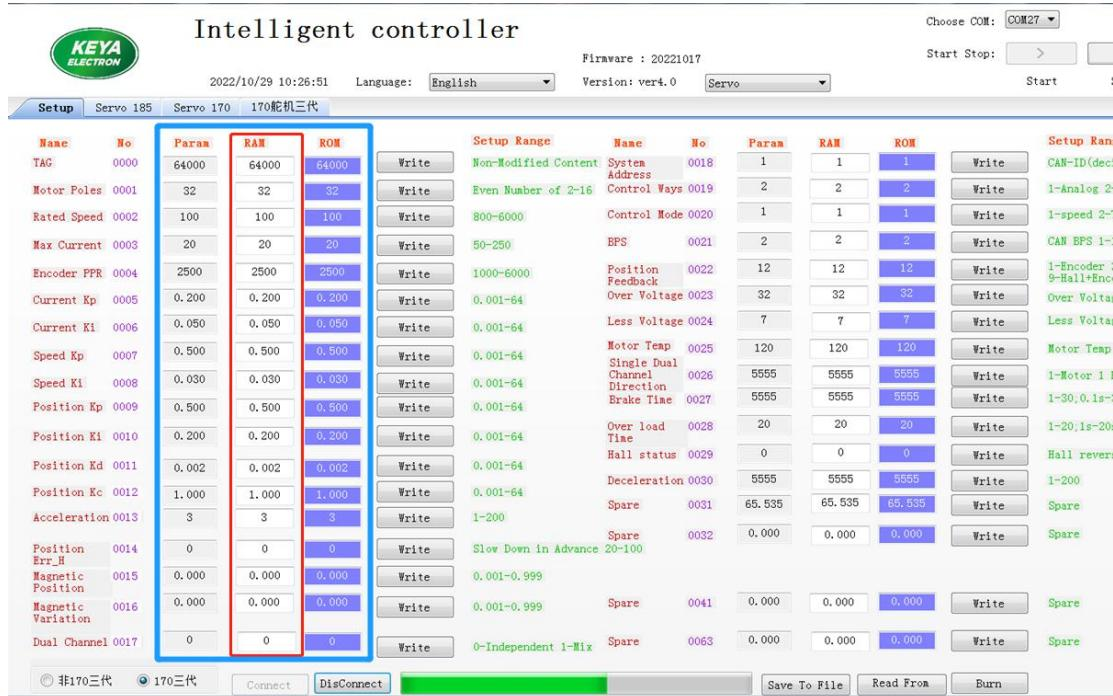
4.1.2.5 For example, if you want modify the number of encoder lines from 48000ppr to 49000ppr, the E<sup>2</sup> ROM data is 48000, please write 49000 in the RAM, and click “Write” button quickly. Confirm that 49000 is no longer changing. Same steps for other parameters, multiple parameters can be modified at the same time.
