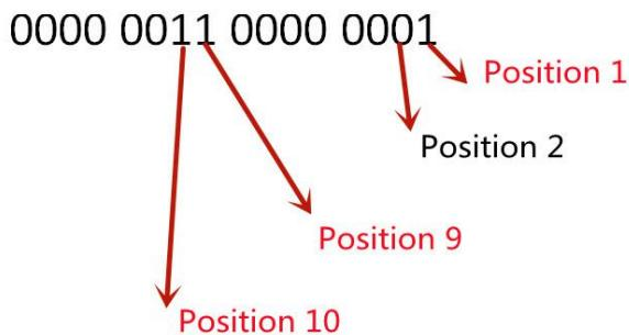
That means three faults : 1, 9, 10
