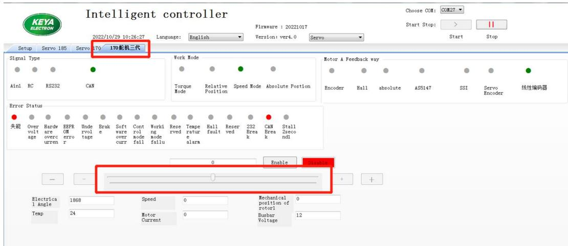
4.1.2.4 The **RAM** in the red box can be modified. The left side of the red box is the controller parameter, and the right side of the red box is the data in the E<sup>2</sup>ROM. In the correct case, the three data are consistent (equal).
