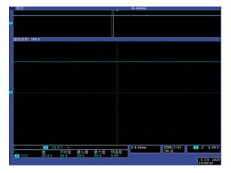
Output dynamic response waveform under 90% ~ 50% load change
