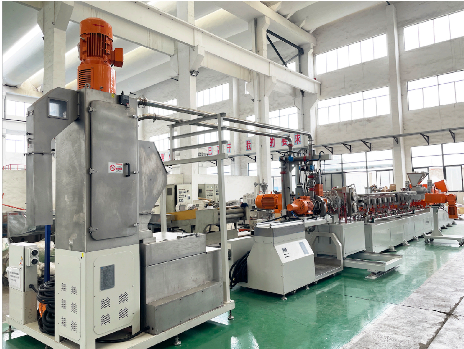
PSHJ-95 Twin screw extruder with underwater pelletizing system for TPE
