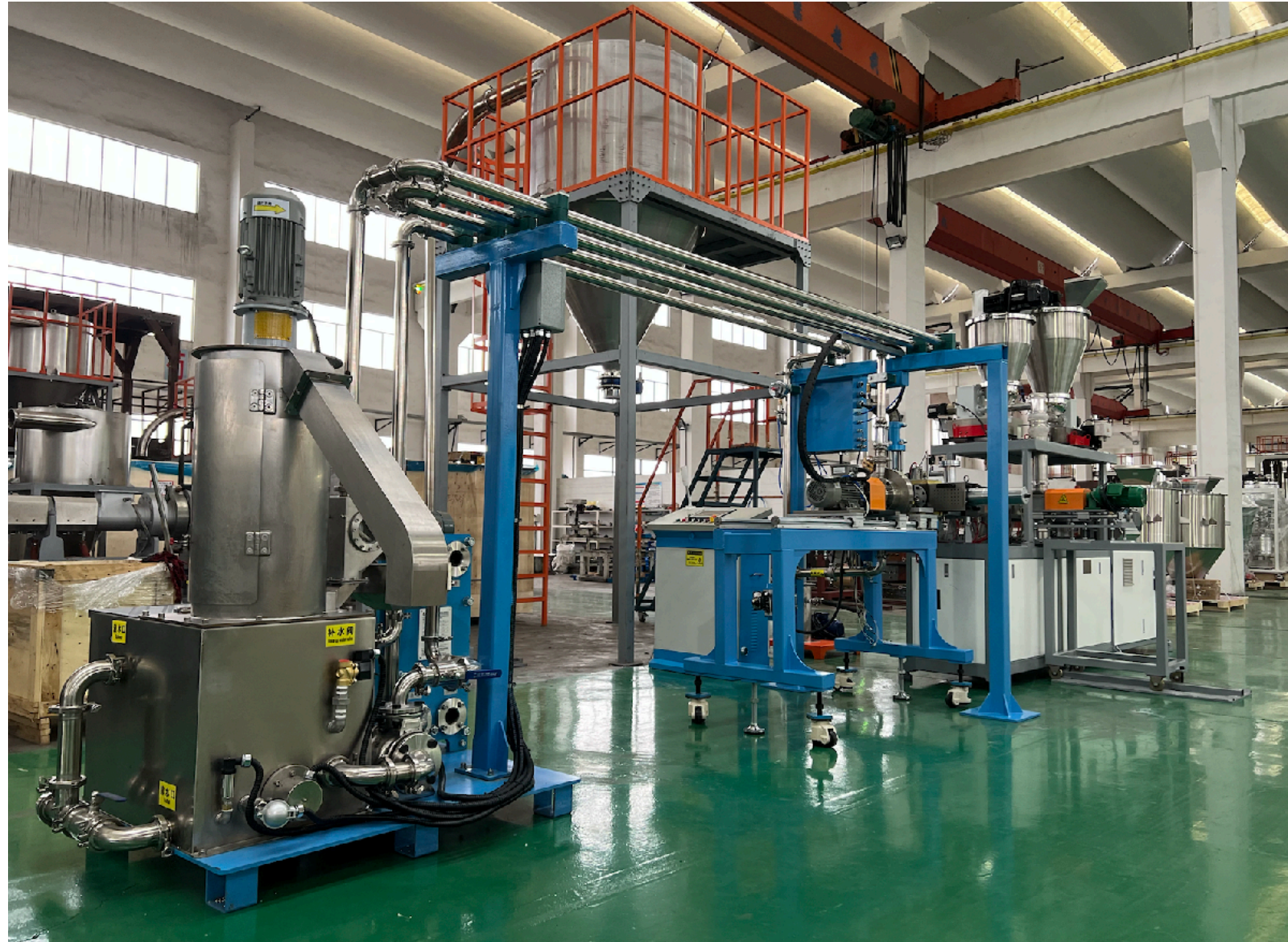
PSHJ-35 Twin scew extruder with underwater pelletizing system for TPU
