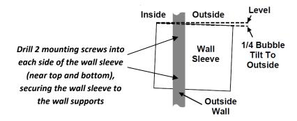
Note\*\* The type of mounting screws used will depend on the type of construction (wood, brick, metal) you are installing the unit through and are <u>not included</u>.
