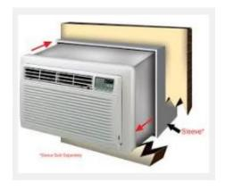
Install included seals between the wall sleeve and the unit. A flat-bladed screw driver or putty knife is recommended to push the seal into the opening between the wall sleeve and unit.
