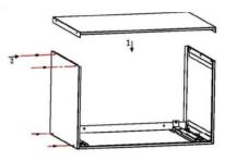
3. As shown in picture 1, install the top cover assembly on top of the left and right cover assembly, and then lock them tightly with screws as shown in picture 2. 2. Cut wall opening to rough-in dimensions of 26-3/16" W x 15-13/16" H x 14-3/4" D max. There must be a minimum 5" clearance to the floor and 24" clearance to the ceiling. (Figure 1) If installed in a concrete or masonry wall, a lintel must be provided in the wall opening for support. (Figure 2)
