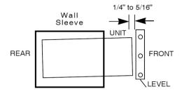
Drill holes in both sides of the side panels (near top and bottom) of the wall sleeve so
