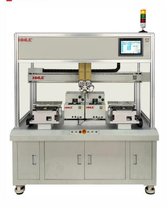
Insert gasket or buckle and then screw. Gasket or buckle of different shapes and materials can be assembled automatically
