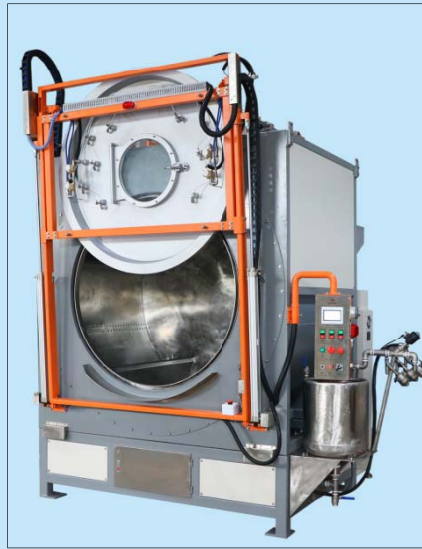
自動門升降裝置，並配備手動檢測門 Automatic front door lifting device, plus a small monitoring window, which can be manually opened
