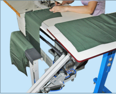
收料架運行工作中 The stacker is working
