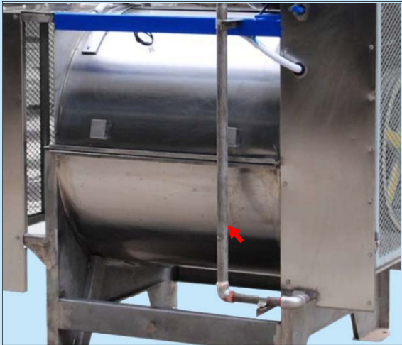
蒸汽直接加溫裝置(NS-2712) Direct steam heating device (NS-2712)
