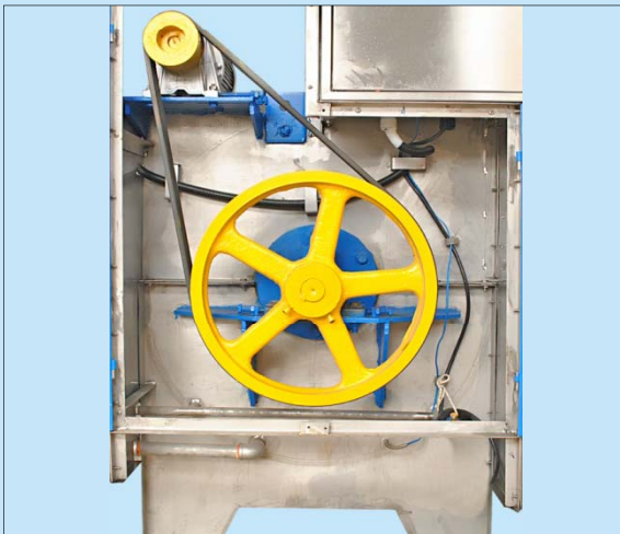
牙箱馬達減速 Speed reduction through gear box
