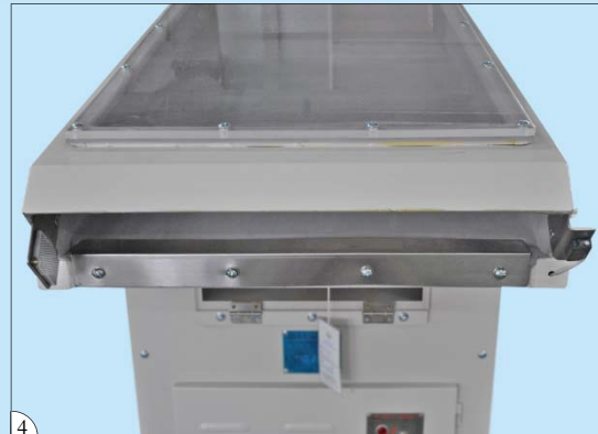
4 NS-55-1電眼感應 Electric eye sensors
