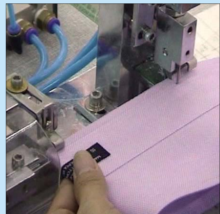
同時在下級領作出刀印及打孔記號 Punch mark applied on collar band simultaneously
