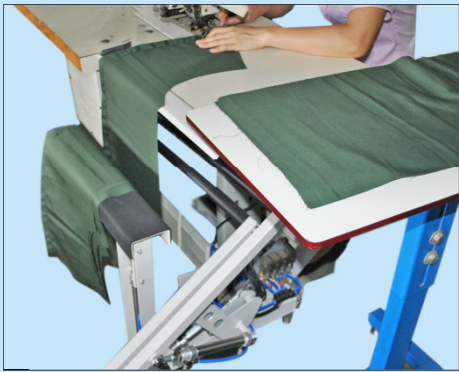
收料架運行工作中 The stacker is in operation
