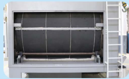
特制加厚保溫裝置，有效減少熱能損耗 Effective heat loss reducing device due to increased thickness of heat insulation layer
