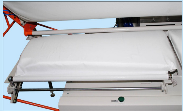
特製壓布框, 可自動拉展褲管 Special fabric clamping frame could stretch and hold trousers' legs automatically so as to get a better pressing effect
