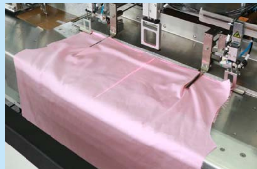
多片裁片一次縫製完成，效率高 Multi cut pieces can be sewn at one stroke, high efficiency
