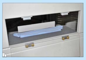
自動收料於操作者前方,取料便捷 Automatic stacking in front of the operator, easy to collect the sleeve plackets
