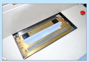
下模抽風便於將裁片折邊、貼合完好 Vacuuming of lower mould facilitates folding and flattening fabric piece
