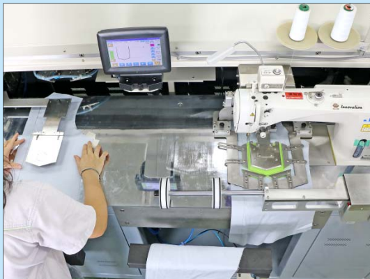
5.機器自動貼袋車縫，同時擺放下件裁片 Automatic pocket sewing while another cut piece being placed
