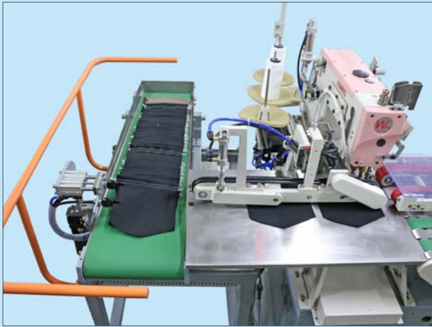
自動縫紉、傳送帶自動收料系統 Automatic sewing, and conveyer belt collecting system
