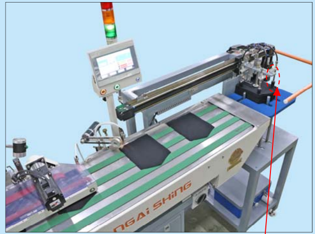
機械手自動上料、輸送、摺邊系統 Robot automatic loading, feeding and folding system
