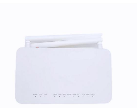
The network side supports downlink 2.488Gbps and uplink 1.244Gbps. The user side provides 4 GE ports, 1 POTS port, 1 USB 2.0 port, Wi-Fi 802.11n 2x2 2.4GHz & 802.11ac 3x3 5GHz concurrently. With the G8670U, home users can access data, video and voice services and enjoy high-speed Internet connections
