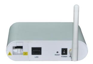
GL-GE8010U-WRtype ONU products fully comply with ITU-T G.984 GPON standards and IEEE802.3ah EPON standards. It is operative, manageable and maintainable at telecommunication level, and can provide high speed data service for customers. It has a PON uplink port that connects to office end apparatus through optical fiber.
